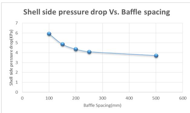
Figure 2. Effect of baffle spacing on shell side pressure drop. (Shell ID = 1.1 m, Baffle cut = 25%, Tube side number of passes = 4, Layout angle = 30°, Tube OD = 19.05 mm, Tube Length = 4.267 m)
