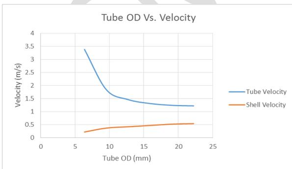
Figure 1. Relation between shell side and tube side fluid velocity and tube OD (Shell ID = 1.1 m, Baffle cut = 25%, Baffle spacing = 0.2 m, Layout angle = 30°, Tube length = 5.486 m)
